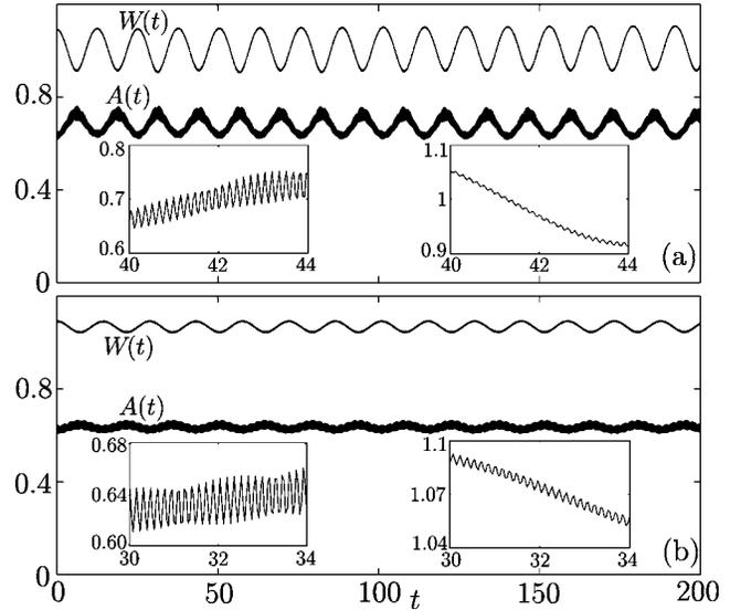
FIG. 1. Evolution of the width  $W = [\int (x^2 + y^2) |u|^2]^{1/2}$  and of the peak amplitude  $A = \max |u|$  of the numerical solution of Eq. (5) for  $n=1$  with a nonlinear coefficient (a)  $g(t) = -2\pi + 8\pi \cos(40t)$ ; (b)  $g(t) = -2\pi + 9.5\pi \cos(40t)$ . Insets show details of the fast oscillations for the amplitude (left panel) and for the width (right panel).
