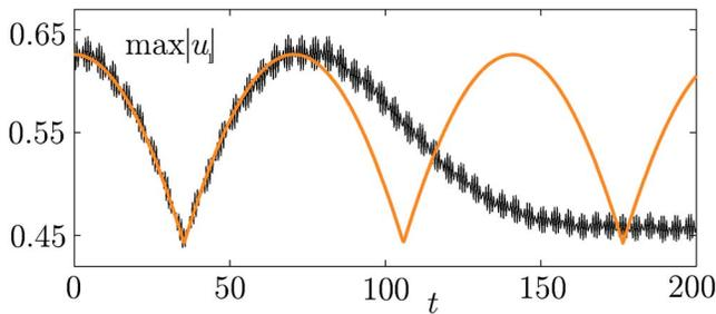
FIG. 10. Comparison of the evolution of the peak amplitude of the wave packet  $u_1$  corresponding to the simulation of Fig. 5 and Fig. 6, obtained by direct numerical simulation of Eq. (5) with the periodic oscillations from Eqs. (31) predicted by the wave packet splitting model.
